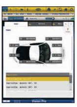
Possibility of connect to a TPMS control unit for its configuration or to assign new sensor codes.
