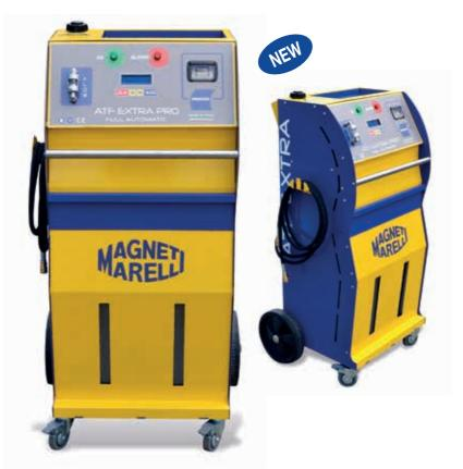
With the **ATF Extra Pro** operator is able to exchange ATF fluid, and flush the automatic transmission in every vehicle. The device has an electronic control system that allows exchanging transmission fluid ATF in an automatic gearbox without opening and complete emptying it, regardless of the temperature difference (and thus the volume) between fresh (cold) and used (warm) transmission oil.
