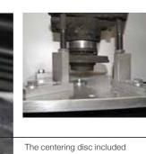
allows you to house the bushings required to remove/insert the silentblock
