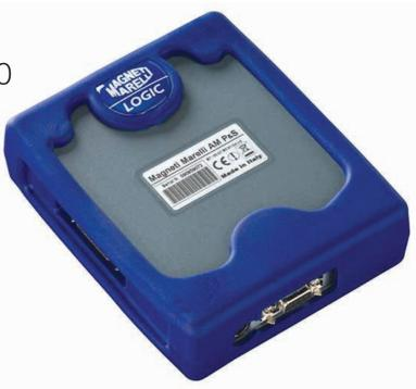
Magneti Marelli Logic - an interface that enables testing of PC-based vehicles. Communication between the cooperating computer and
