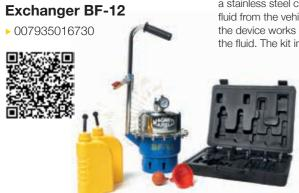
Universal pneumatic device for brake fluid replacement. The device consists of a stainless steel container, inside which a rubber diaphragm moves, sucking the brake fluid from the vehicle. After filling the internal tank to maximum operating pressure, the device works independently. Just one technician is required to completely replace the fluid. The kit includes service adapters, hoses and two 1-litre reservoirs.
